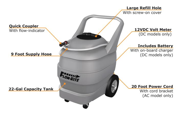
The AC & DC portable watering cars are ruggedly constructed of lightweight yet strong polyethelene plastic, and features a large 22 gallon holding capacity. The new cart also features a large refill hole with screw-on cover to keep out particles. A 12-volt sealed battery with its own on-board charger power the DC watering cart's variable speed pump. All components are DI water compatible.
